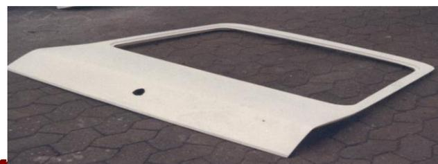
Heckklappe GFK Standart
